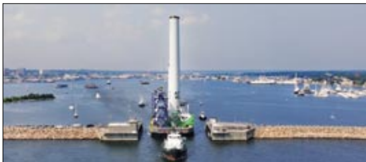
Tugboats move a 400-foot barge through the New Bedford Hurricane Barrier gate on 9/6/23 that is carrying components of offshore wind turbines for Vineyard Wind's project 30 miles off the coast of Cape Cod, including three 321-foot turbine blades, and parts of the tower that will be 700 feet tall when fully constructed/assembled offshore. Submitted photos.
